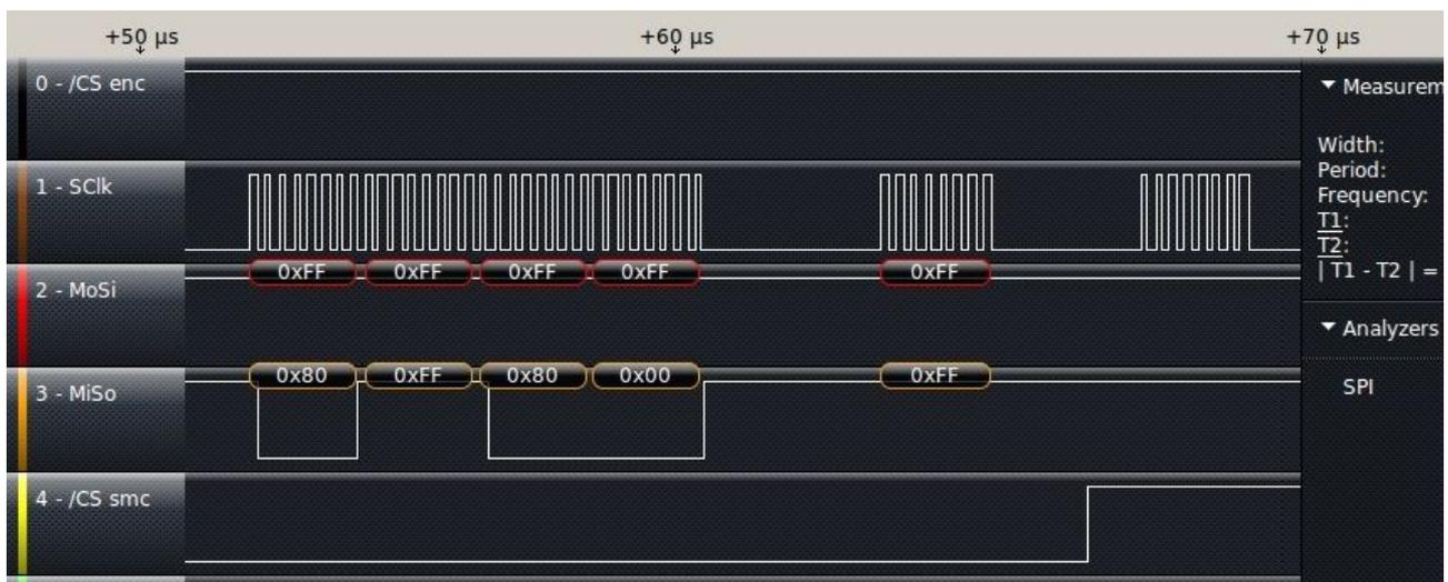
Figure 4: Part of a Saleae Logic screen shot (tracing SPI communication)
