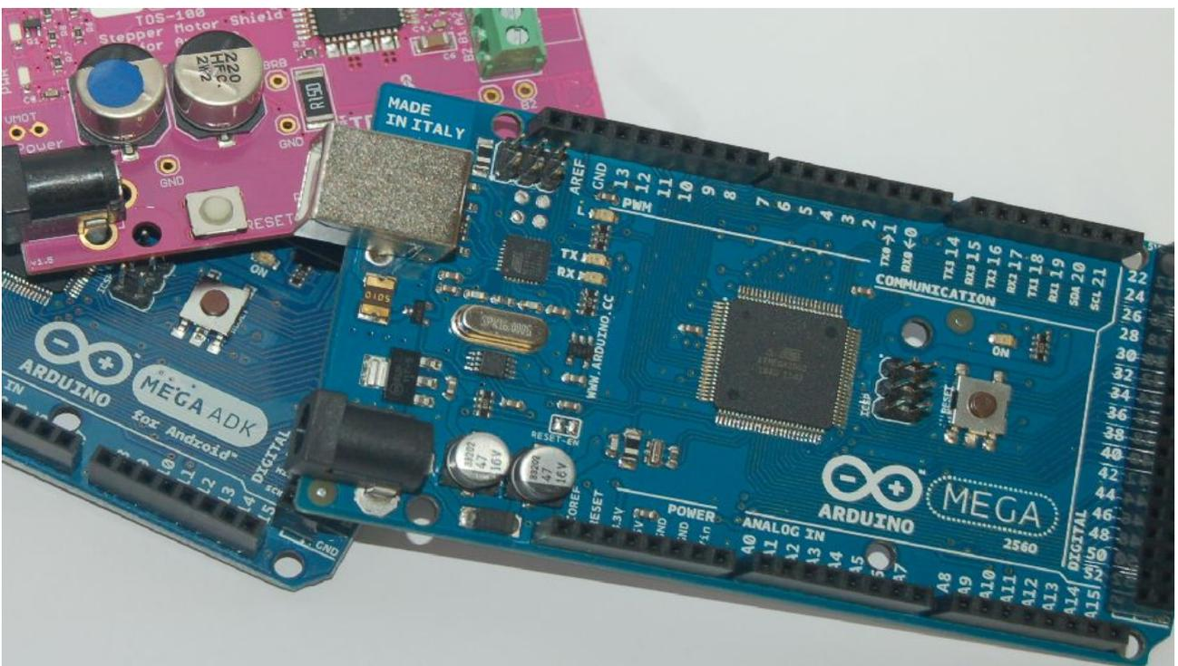
Figure 2: The ArduinoMega2560 (top), the ArduinoMegaADK (covered) and a “shield” (pink)
